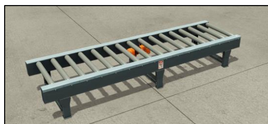
Figure 5.3 - Roller Conveyor available in the previous Factory IO edition
