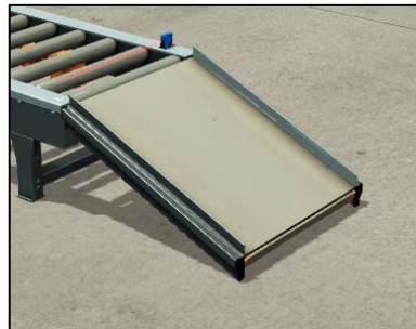
Figure 5.14 - Low Chute Conveyor
