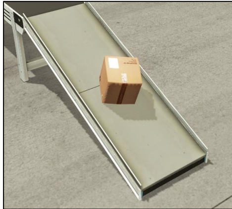
Figure 4.6 - Chute Conveyor dispatching an item
